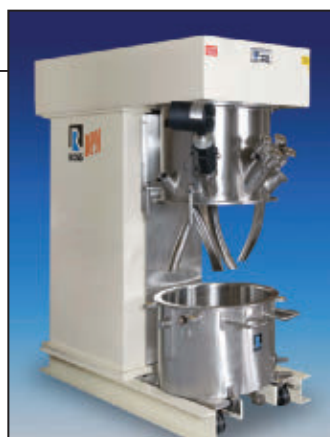
FIGURE 3. Equipped with helical blades, the double planetary mixer’s operating viscosity range is extended from approximately 2 million cP to at least 8 million cP. The mixer’s ability to disperse powders rapidly is also dramatically improved. As the helical blades advance, they continuously push powders forward, down and inward
